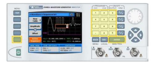
Enter the number of the sequence to be edited and press **ENTER**. Up to 10 sequences can be stored in the system, recalled, and replayed\*.
